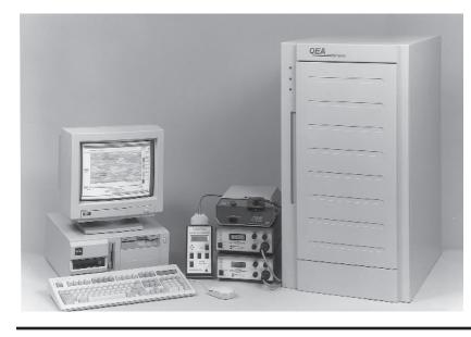
The PDT-1000 is a computer-controlled multifunction test system for evaluating photoreceptors used in electrophotographic printers and copiers. This flexible system accommodates a wide range of drum types and sizes and performs many types of tests including surface mapping, electrophotographic characterization, coating uniformity measurement, and substrate cleanliness evaluation.
