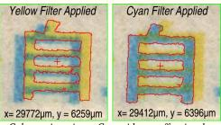
• Color registration: Centroids are offset in x by 360μm and in y by 137μm.
