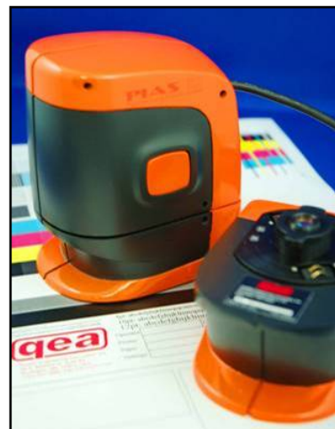
Fig. 1 The PIAS-II with an optional optical head in the foreground. Dimensions of the main unit are approx. 100mm (H) x 80mm (D) x 60mm (W).
