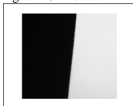
Fig.6 Example image featuring a “slanted edge”
