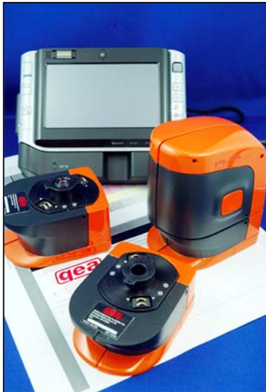
Figure 2. Portable image analysis system (right) shown with two optional optics modules (left and front) and an ultra-compact computer.
