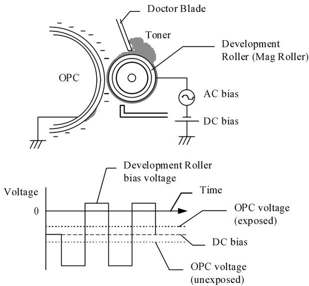
Figure 1. Developing an Image on the OPC in a Magnetic Monocomponent Development System
