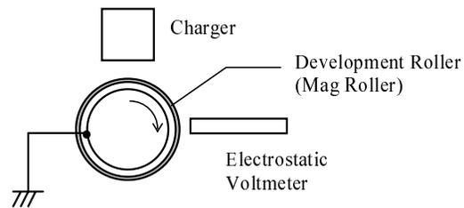
Figure 2. Schematic of Electrostatic Charge Decay Measurement
