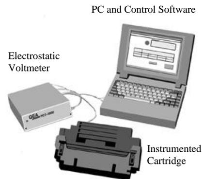
Figure 2: A Basic Instrumented Cartridge Test System
