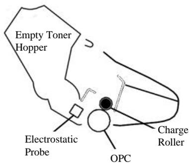
Figure 1: Schematic Diagram of an Instrumented Cartridge
