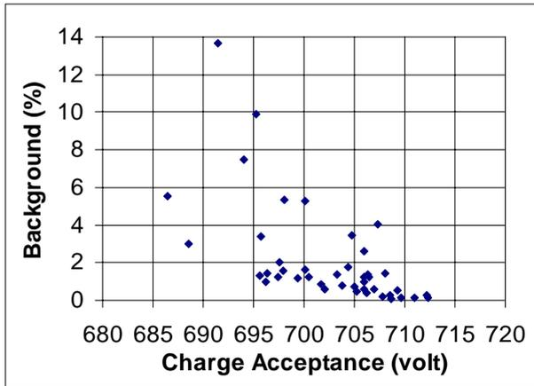
**Figure 8: Correlation Between Charge and Background in Print Tests of the Two-Cycle Used OPC Samples**
