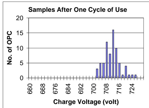
Figure 3: Charge Voltage Distribution for One-Cycle Used OPCs
