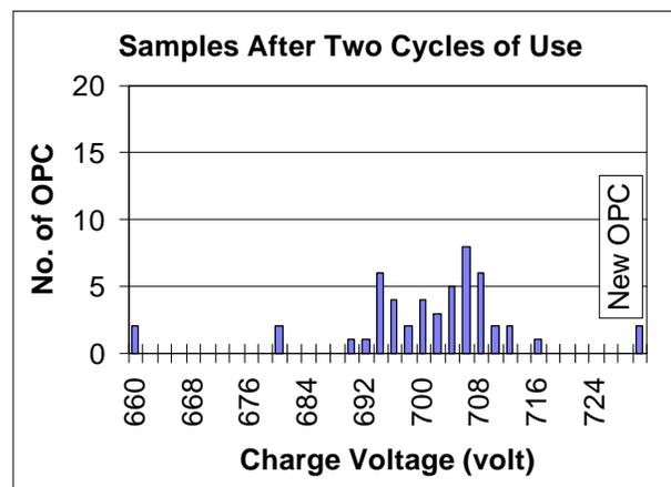
Figure 4: Charge Voltage Distribution for Two-Cycle Used OPCs
