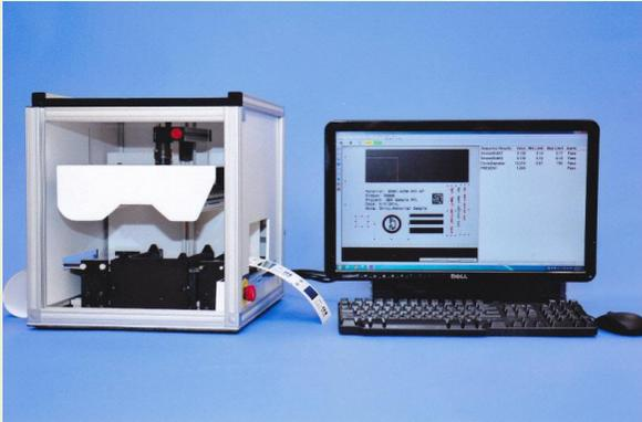
The IAS-1000L is an automated label print quality analysis system ideally equipped to analyze strips or continuous rolls of labels in a broad range of sizes. Performing objective measurements automatically, efficiently and consistently, it eliminates the need for subjective visual inspection and tedious manual measurements.
