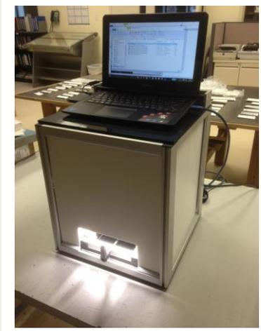
The IAS-3000P is a print quality analysis system designed specifically for quality sampling in a production environment. At the touch of a button, the system performs objective measurements on labels, cards, or other samples up to about 4" x 6" inches, eliminating the need for subjective visual inspection and manual measurements.
