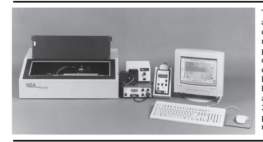
The PDT-2000LTM is an advanced drum test system for characterization of photoreceptors used in electrophotographic printers and copiers. Designed primarily for drum testing, the system can also be used for sheet sample testing by wrapping the test sample around a bare drum. The PDT-2000LTM is typically used in production quality control and in research and development.
