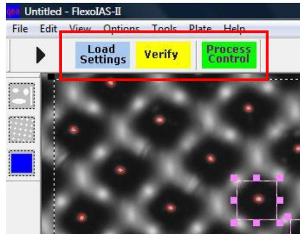
Fig. 4b Process Control (Programmed Sequence Measurement) Tools (FlexoIAS-IIPC and FlexoIAS-IIPCP only)
