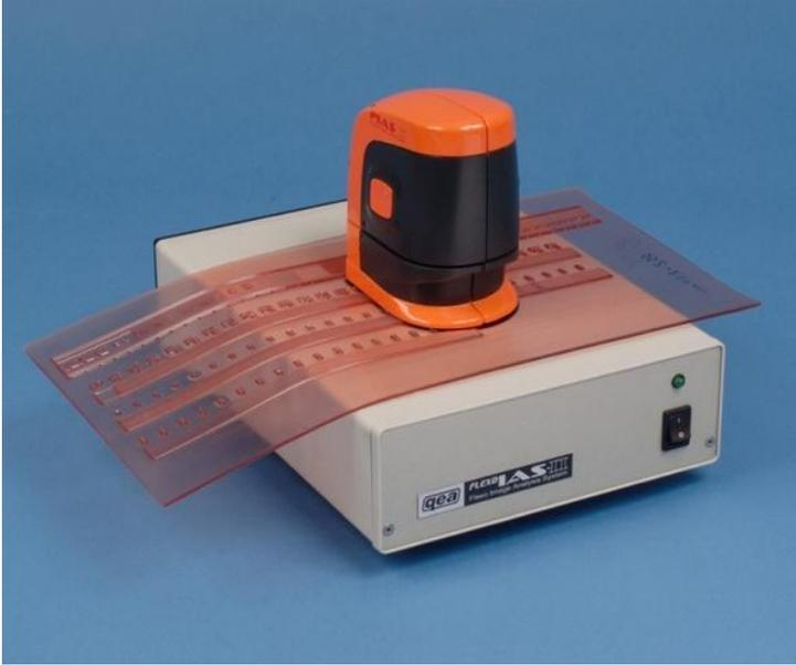
Fig. 10. FlexoIAS-II without optional control strip guide.
