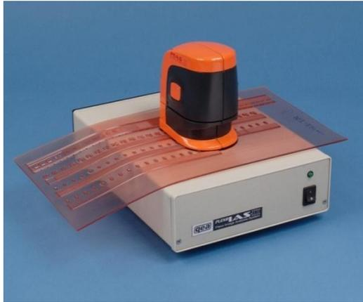
Fig. 2a. FlexoIAS-II Measurement Unit and Light Box with test sample
