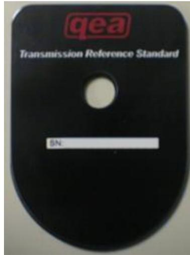
Fig. 7 *Transmission Reference Standard* for system calibration and performance verification
