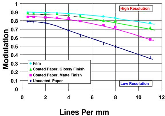
Figure 10: Effect of Media Type on Modulation (Resolution)
