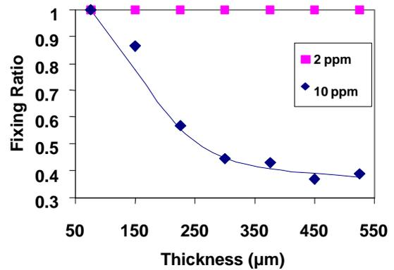
Figure 5: Effect of Paper Thickness on Fusing Quality at Two Fusing Speeds
