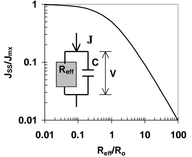
Figure 4. Variation of steady state currents  $J_{SS}$  with the effective resistance  $R_{eff}$ , Eq. (8).  $J_{SS}$  and  $R_{eff}$  are normalized to the units  $J_{mx}$  and  $R_o$ , respectively, defined in Eq.(3). The inset shows the equivalent circuit for the steady state under corona charging.
